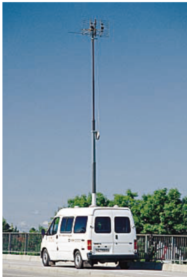
FIG 2 Test vehicle with Spectrum Monitoring System for Broadcast Applications SMSB Photo 42 882/2
