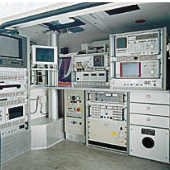
FIG 1 Vehicle-mounted Spectrum Monitoring System for Broadcast Applications SMSB Photo 42 882/3
