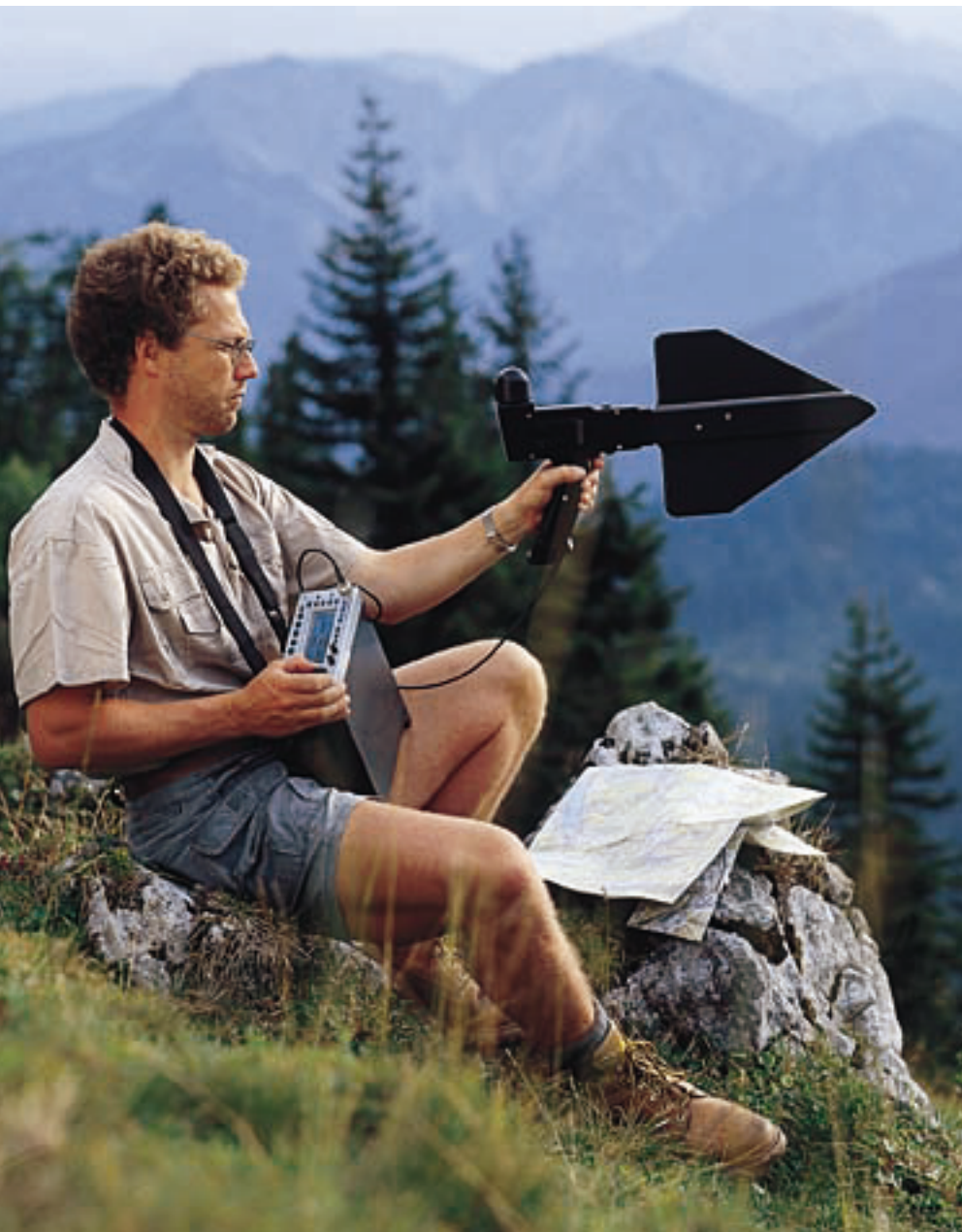
FIG 1 With a weight as little as 4 kg, Miniport Receiver EB200 can conveniently be carried and operated, leaving one hand free for Directional Antenna HE200. Photo 43 016/1
