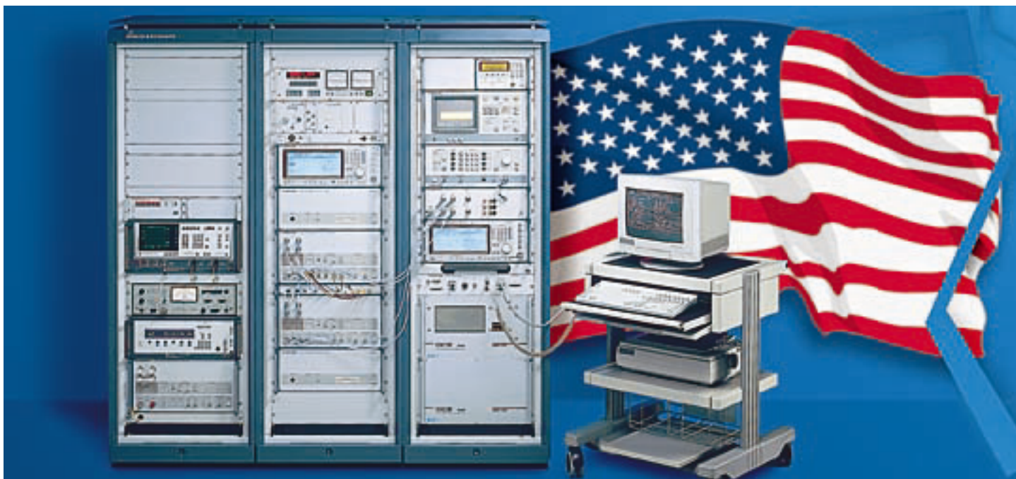
FIG 1 PCS1900 System Simulator TS8915 provides more than 200 test cases for type certification of US mobile phones to PCS1900 standard.
